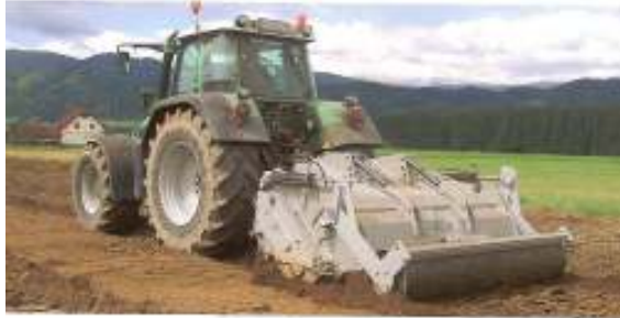
Recultivation with rotary cultivator – rotary brushwood chopper
