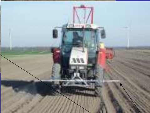
Plot sprayer with special spray booms and band spraying
